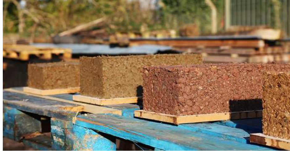
Image above: Digero Compressed Structural Blocks drying in the sun.
