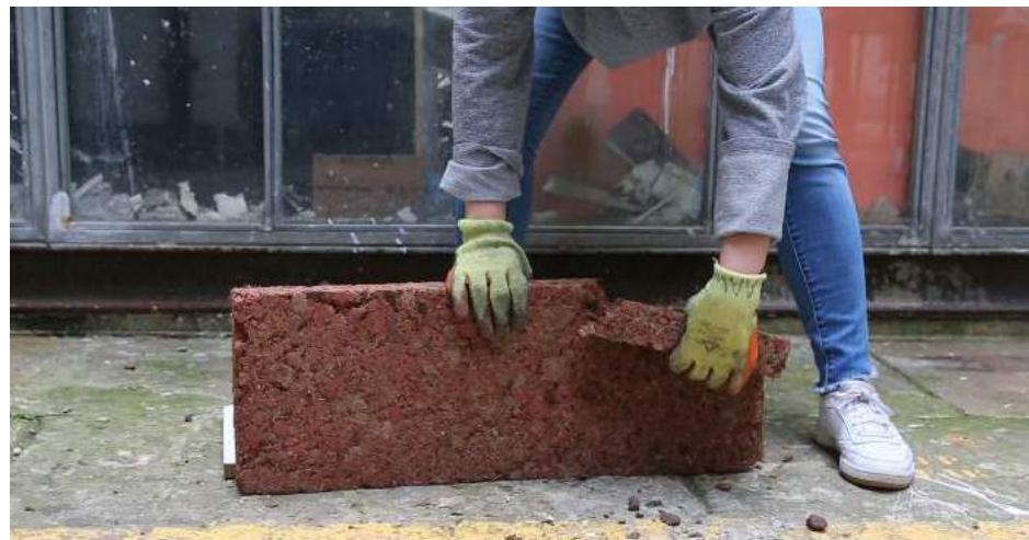
Image above and below: Digerio Compressed Structural Panels undergoing strength testing.
