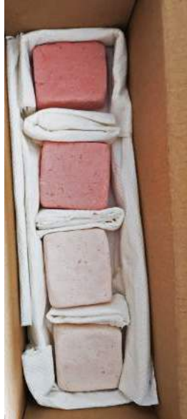
Images above: Testing sample bricks for various chemical bonding ratios.
